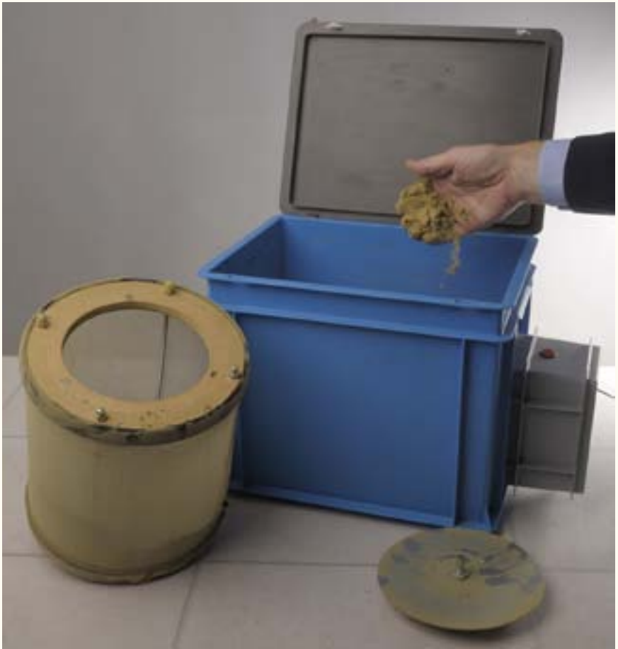
Figure 1.9: A so-called pollinator device, used to collect trichomes from dry cannabis herbal material
